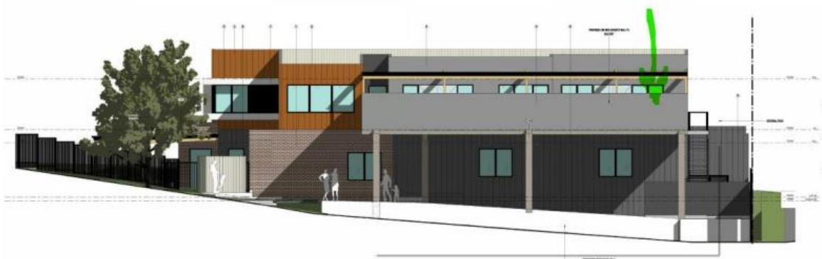
Figure 11- Elevation including balcony acoustic wall.
